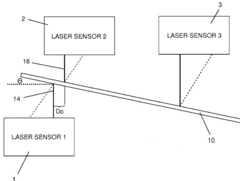
The above diagram from our U.S. Patent #9,151,595 shows the need to correct for lack of laser beam collinearity. The following formula is used in these cases.
